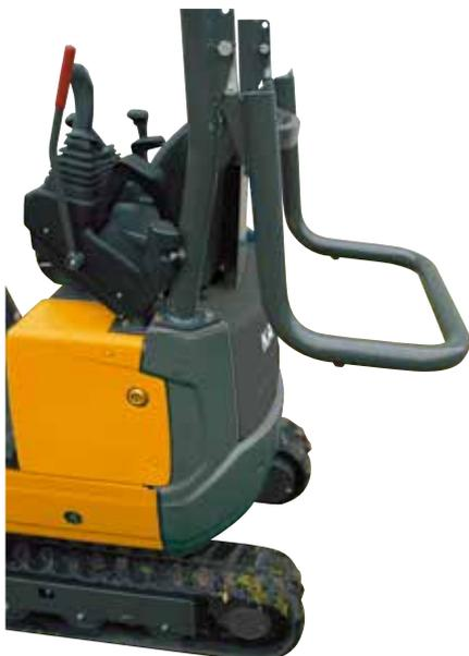
The HD12VXE can drive through doors no more than 90 cm wide. The rollbar can also be removed in just a few minutes to facilitate passing through low clearance areas.
